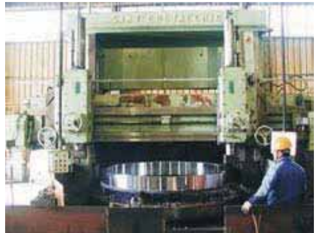
VERTICAL LATHE M/C (Subsidiary DKMC) SIZE : 6,000 \varnothing x 1,600H
