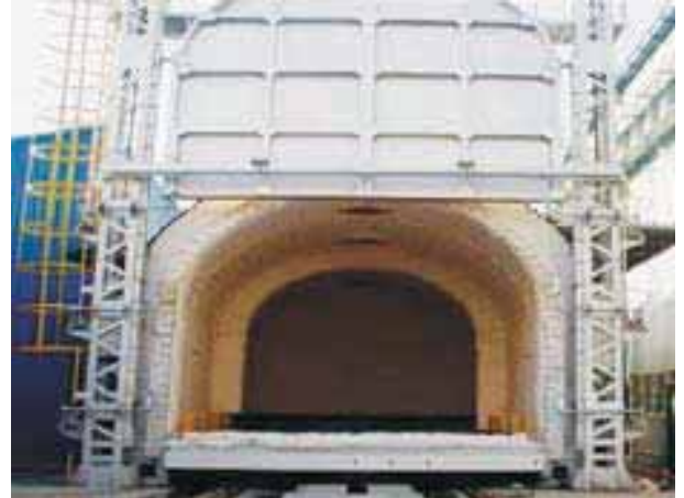
FURNACE (P.W.H.T & S.R) SIZE : 13,000L x 4,350W x 4,600H (mm)
