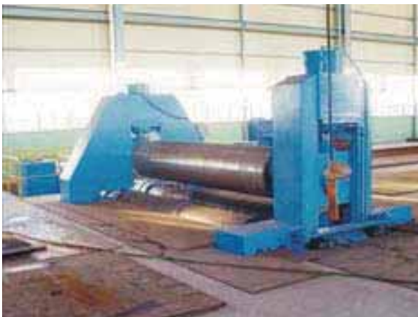
3 ROLL BENDING MACHINE (Capacity : Max. Th'k 50mm / W 4,000mm)
